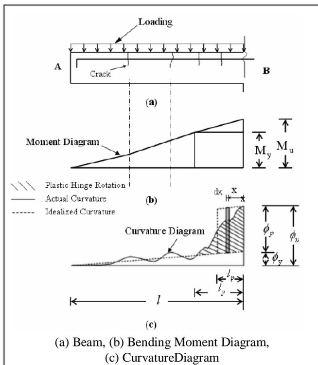
Fig. 3 Schematic Curvature Distribution along Beam at Ultimate Stage.
