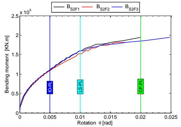
Fig. 6 Moment- rotation relations developed in the beams of RC frame (Beams of 2<sup>nd</sup> level).
