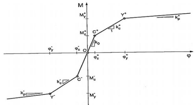
Fig. 2 Moment-curvature response of modified TAKEDA model [16].
