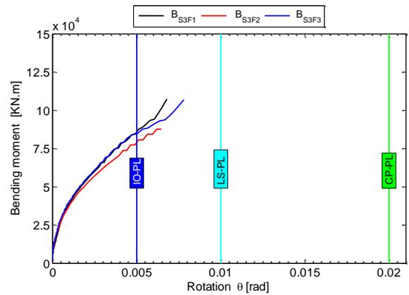
Fig. 7 Moment- rotation relations developed in the beams of RC frame (Beams of 3<sup>rd</sup> level).
