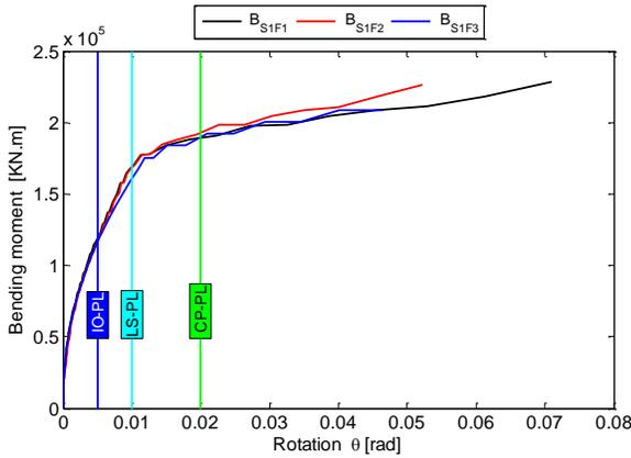
Fig. 5 Moment- rotation relations developed in the beams of RC frame (Beams of the 1<sup>st</sup> level).
